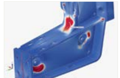
The optimized design with welded inserts using Inspire.
